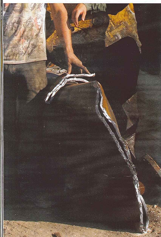
Hlh&r shows how their Allied-Gator MTR 90 S powers through heavy-wall pipe.
